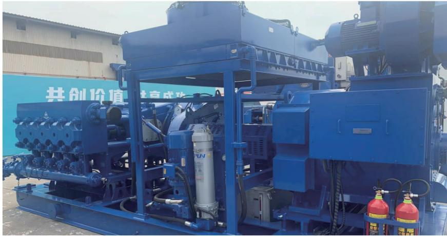
HH6000R電動壓裂泵
