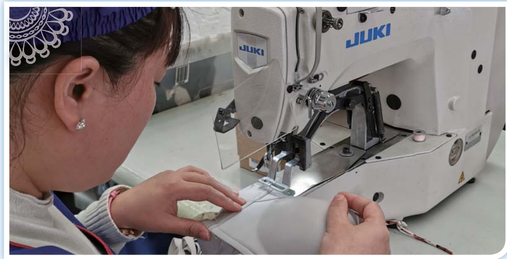
A baffle is installed on the sewing machine to prevent the broken needle from splashing into the eyes. 衣車上安裝防斷針飛濺傷眼的擋板，以防斷針彈出。
